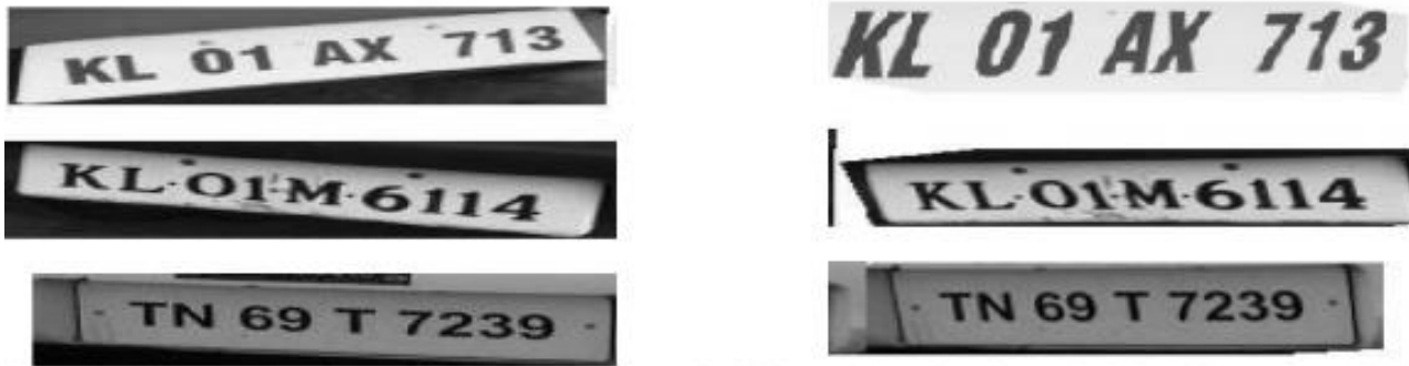
Skewed vehicle number plates (left) and Skew corrected vehicle number plates by using Hough Transform (right)
